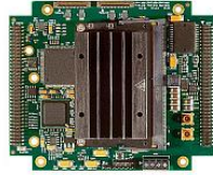
JetStream Multi-Channel Video AI Carrier Board
