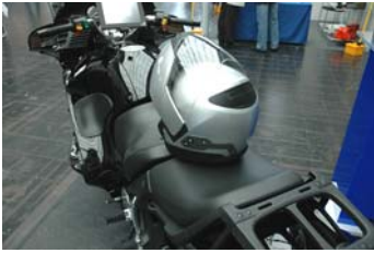
BMW-RT with DeltaCar-PC und helmet with BlueTooth-handsfree set (2 microphones, 2 speakers are integrated in the helmet)
