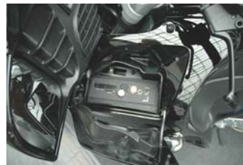
Installation situation of the DeltaCar PC in the DIN pit housing of motorcycle BMW-RT
