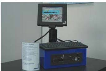
DeltaCar-PC with 6,5" LCD-TFT-monitor and software-solution for navigation (Moving Map) for general aviation
